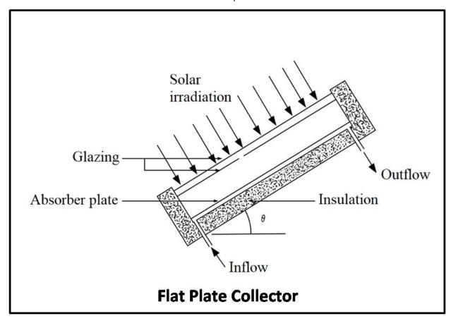
In the plate collector, the solar radiation is absorbed by the plate having black surface and then absorbed heat get transferred to the fluid/air filled in the tubes. The thermal insulation in the bottom and sides of the collector, and the glass screen above the plate prevents heat loss during transfer of heat.
